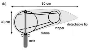
Fig. 2. (a) Picture of an experimental windsock in the field; (b) detailed schematic drawing illustrating the design of the experimental wind socks. Essential parts such as the zipper to detach the tip of the sock and the metal frame used to keep the mouth of the wind sock open at all times are indicated.
